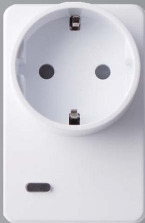
The PSMD-29ZW power meter plus dimmer switch is designed for the user to remotely dim or turn on/off incandescent light via a smartphone or tablet anytime, anywhere. The PSMD-29ZW has a built-in power meter to measure electricity consumption, allowing users to conveniently control home lighting for comfort and energy-saving purposes.
